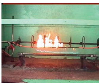
FIRE TEST CATEGORY C
