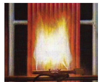
CABLES DURING IEC 60332 PART 3 TEST
